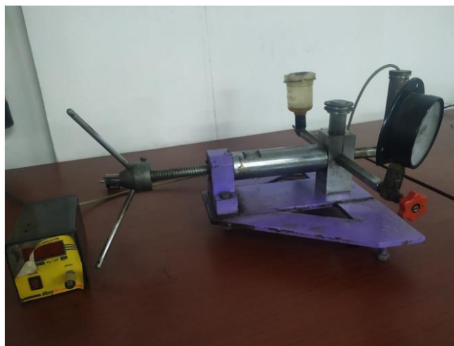
Fig. 6.1 : Schematic showing pressure gauge based load pressure testing.
